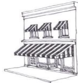
This figure illustrates more appropriate awnings that fit the original window openings and does not obscure view of the architectural features. The lower awning is at a 30-45 degree angle, and has a 6-8" loose valance, and the lower edge of the awning is 7 feet above the ground. The upper awnings have a 45 degree angle, fit the opening width of the window and extends the half way point of the opening height.
