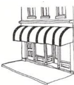
This figure illustrates an inappropriate awning. The awning spans from building edge to building edge exceeding the size of the original window. Additionally, the awning does not have a valance, the entire awning is rigid/fixed and it is a bubble style awning.
